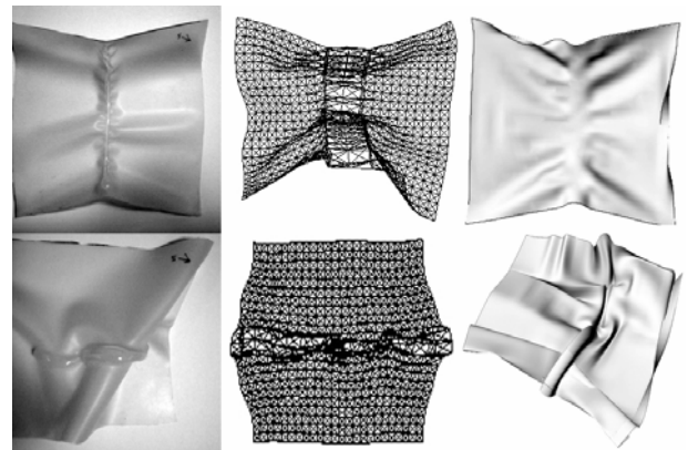
Fig 3 Real-time digital simulation (in the Processing environment) of resin impregnation as applied perpendicular (top) and parallel (bottom) to the stretch resulting in sewed-like creases and directional folds respectively.
