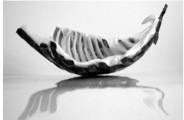
Fig 2 Resin impregnated latex membrane demonstrating curvature induced by pre-stretching.
