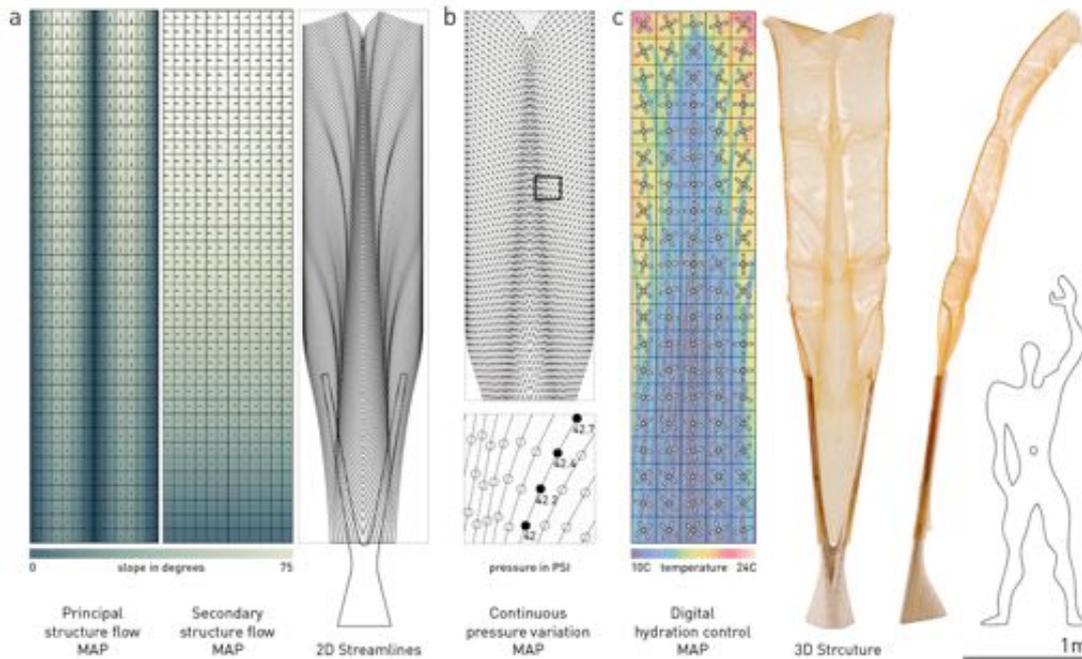
**Figure 5:** (a) Vector fields encode variation in principal and secondary structure, and are interpolated into streamlines of material deposition trajectories. (b) Pressure, speed and material concentration variation along structural streamlines is encoded into real-time instructions sent to the manufacturing platforms. (c) Computerized hydration control maps on top of deposited structures provide global evaporation-driven self-folding of the final functional 3D structure.
