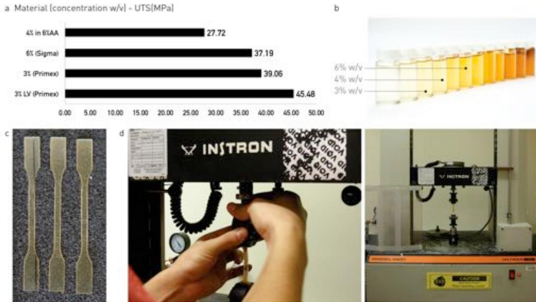
**Figure 2:** (a) Ultimate Tensile Strength (UTS) testing results of chitosan film dogbones in different concentrations and purchased from different companies (b) Chitosan concentrations in gel state (c) 3D printed and laser cut dogbones before being tested (d) Instron mechanical tester with a 9071.85kg reversible load cell.
