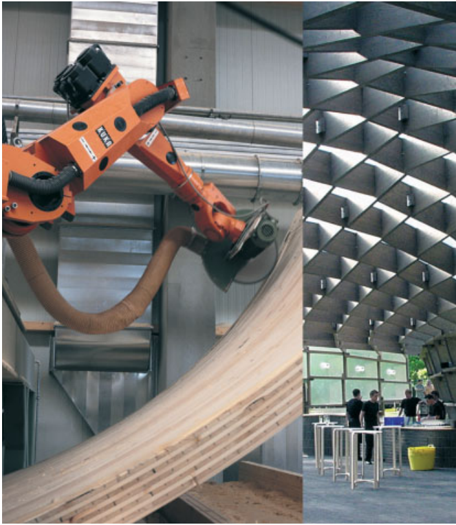
Robotic timber-manufacturing employed for the 2005 Serpentine Pavilion, as discussed in 'Manufacturing Diversity' (see page 70).
