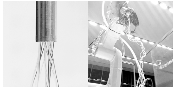
Figure 6a. (L.) Multi-strand HDPE extrusion close up. Figure 6b. (R.) Multi-strand HDPE extrusion in space.
