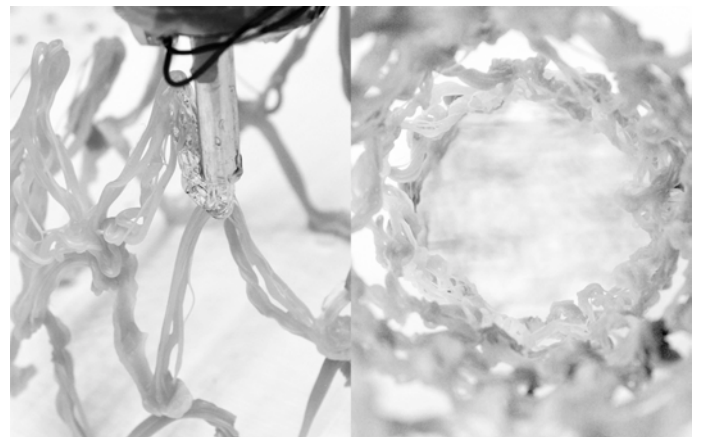
Figure 7a. (L.) Close-up of HDPE freeform prototype. Figure 7b. (R.) Detail of finished HDPE freeform prototype.
