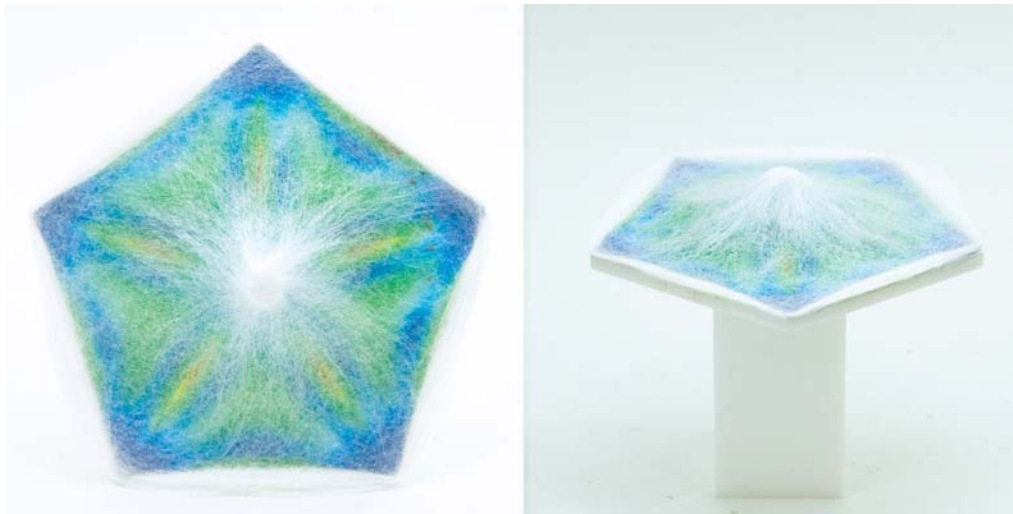
Figure 10 One-dice polygonal platforms showing greater density of silk deposition in areas of higher Stress-Strain.
