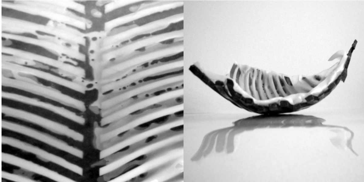
Fig. 2 Resin - impregnated latex membrane model demonstrating curvature induced by pre-stretching, shown in two scales.
