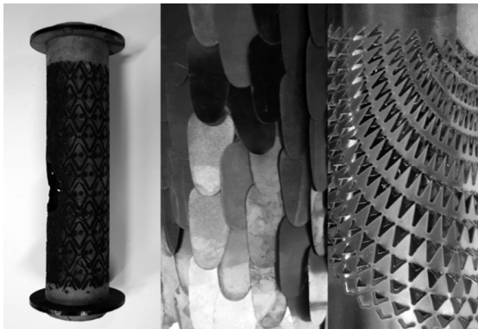
Fig. 4 Rotary laser-cutting as a form of "digital lathing". Left: mandrill designed to support cylindrical acrylic structure; Middle and right: acrylic structure with water-jet cut scale-like elements attached in additive (middle) and subtractive (right) methods.
